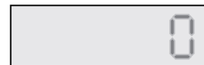
Fig. 6a: Upon startup for the -EC models, counter should read zero. If a non-zero is displayed, the counter can be reset by following Step 6. If the counter is blank, contact MCG Support at 1-800-851-1508.
