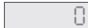
Fig. 5a: Upon startup for the PT250 and -EC models, counter should read zero. If a non-zero is displayed, the counter can be reset by following Step 6. If the counter is blank, contact MCG Support at 1-800-851-1508.
